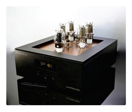
Pacific 3 has all the elements that constitute an ultra audiophile product: zero feedback design, zero silicon design (in signal path) latest and best digital conversion technology, tube rectified power supply, active tube anode loading, Directly Heated Triodes output stage in single-ended scheme, copper sheet capacitors, and many other features designed with one thing in mind – pure music.
